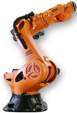
(b) Example of Serial Manipulator (KUKA Robotics Cooperation)
