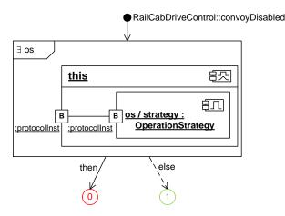
Figure A.84: Component SDD convoyDisabled for Component RailCabDriveControl that Specifies that an Instance of the Component will not Engage in Convoys
