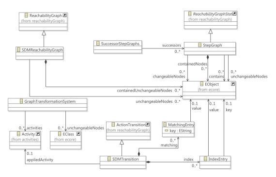
Figure C.3: Class Diagram of the Metamodel for Reachability Analysis on Story Diagrams
