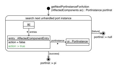
Figure A.78: Story Diagram Specifying the Behavior of getNextPortInstanceForAction
