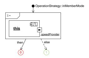
Figure A.91: Component SDD inMemberMode for Component OperationStrategy for Specifying that an Instance of the Component Operates in a Member RailCab
