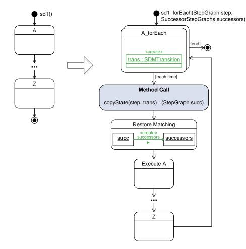
Figure C.4: Enhancing Story Diagrams for Computing Successors
