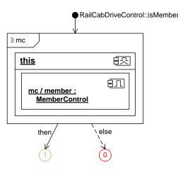
Figure A.83: Component SDD isMember for Component RailCabDriveControl that Specifies that an Instance of the Component Operates as a Convoy Member
