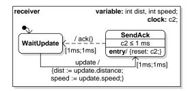
Figure 2.14: RTSC of Role receiver of DistanceTransmission
