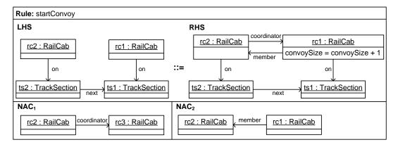
Figure 2.8: Graph Transformation Rule for Starting a Convoy
