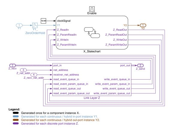
Figure 6.7: Generation Template for Creating the Internal Structure of a Subsystem for an Atomic Component Instance
