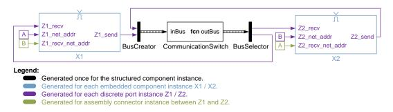
Figure 6.14: Generation Template for Translating Assembly Connector Instances
