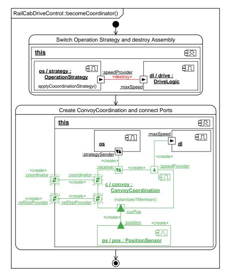
Figure A.53: CSD for Component RailCabDriveControl that Reconfigures the Component Instance to Serve as a Coordinator
