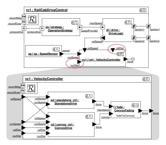
Figure 4.7: Problems when Replacing Continuous Component Instances using Singe-Phase Execution
