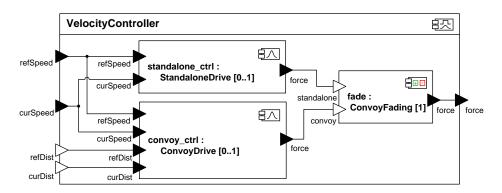
Figure 3.7: The component type VelocityController
