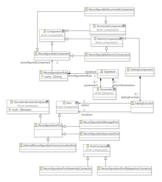
Figure D.6: Class Diagram of the Metamodel for Reconfigurable Components
