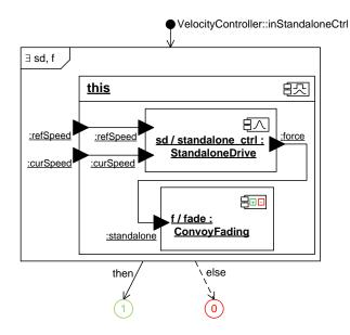
Figure A.87: Component SDD inStandaloneCtrl for Component VelocityController for Specifying that an Instance of the Component Executes the StandaloneDrive Controller
