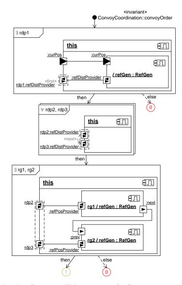
Figure A.86: Invariant Component SDD convoyOrder for Component ConvoyCoordination for Specifying a Correct Order of the RefGen Instances
