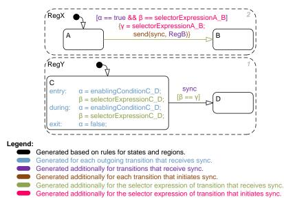
Figure 6.21: Generation Template for Translating Transitions with Synchronizations with Selectors to Stateflow
