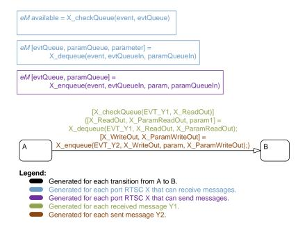
Figure 6.17: Generation Template for Translating Sent and Received Messages of Transitions to Stateflow
