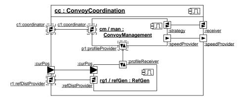
Figure A.29: Component Instance of Component ConvoyCoordination for a Convoy with 1 Member
