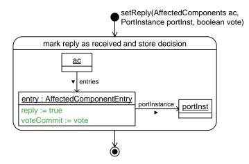
Figure A.75: Story Diagram Specifying the Behavior of setReply
