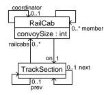
Figure 2.6: Example of a Type Graph
