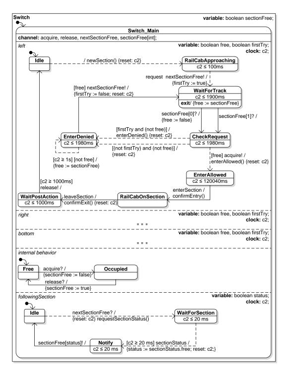
Figure A.40: RTSC of the Component Switch
