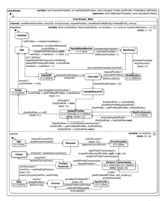
Figure A.4: RTSC of the Role coordinator of the RTCP ConvoyCoordination (cf. [FHK<sup>+</sup>14])
