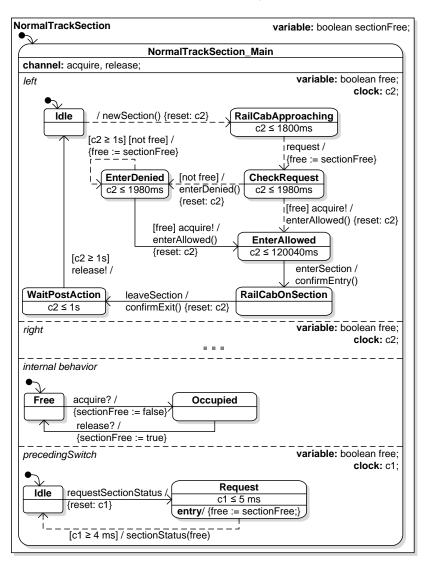
Figure A.39: RTSC of the Component NormalTrackSection
