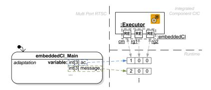
Figure 6.29: Array Implementation of the AffectedComponents Structure
