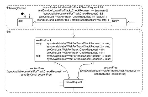
Figure 6.22: Example of Using Transitions with Synchronizations with Selectors in Stateflow
