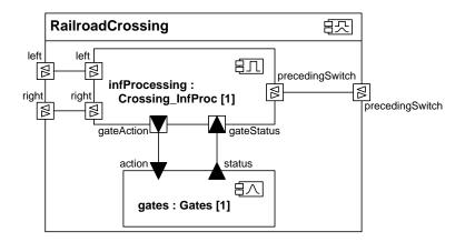
Figure A.26: Structured Component RailroadCrossing
