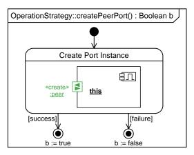
Figure A.66: CSD for Component OperationStrategy that Creates a peer Port Instance
