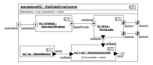
Figure 3.9: Component Instance of Component RailCabDriveControl for a RailCab Driving Alone
