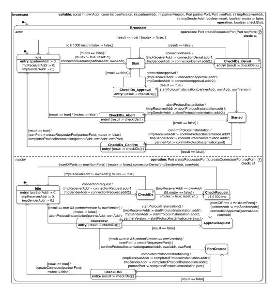
Figure A.23: RTSC Implementing the Broadcast Communication for Instantiating the RTCP ProtocolInstantiation
