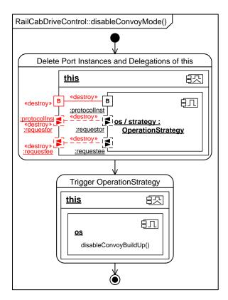
Figure A.60: CSD for Component RailCabDriveControl that Disables the Convoy Mode by Deleting the Necessary Port Instances for Convoy Build-up
