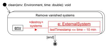
Figure A.22: Story Diagram Implementing the Operation clean
