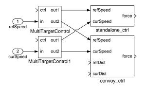
Figure 6.13: Example for Using a MultiTargetControl Block for Translating a Reconfigurable Delegation Connector
