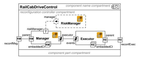
Figure 4.2: Reconfiguration Controller of a Structured Component (cf. [HB13])
