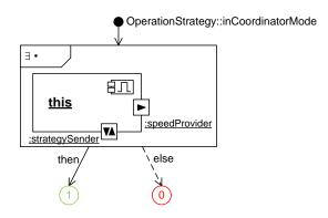
Figure A.90: Component SDD inCoordinatorMode for Component OperationStrategy for Specifying that an Instance of the Component Operates in a Coordinator RailCab
