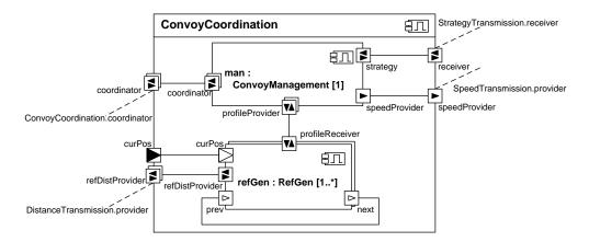
Figure 3.5: The structured component type ConvoyCoordination
