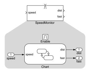
Figure 6.2: Enabled Subsystem
