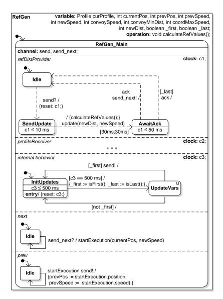
Figure A.38: RTSC of the Component RefGen
