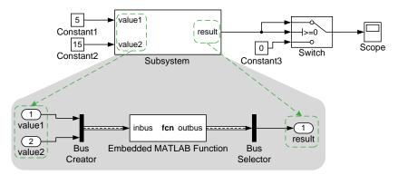
Figure 6.1: Simple Simulink Model
