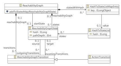
Figure C.2: Class Diagram of the Core Metamodel of the Reachability Analysis Framework
