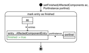
Figure A.80: Story Diagram Specifying the Behavior of setFinished
