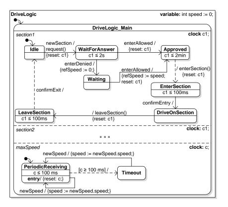
Figure A.35: RTSC of the Component DriveLogic
