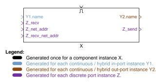
Figure 6.6: Generation Template for Creating a Subsystem for an Atomic Component Instance
