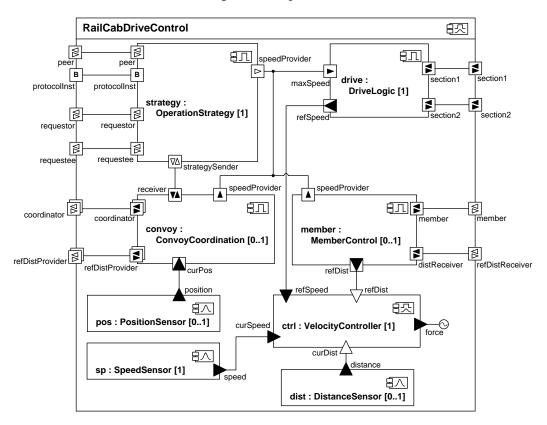
Figure 3.6: The component type RailCabDriveControl
