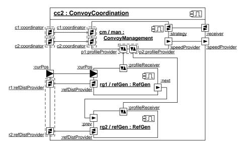
Figure A.30: Component Instance of Component ConvoyCoordination for a Convoy with 2 Members
