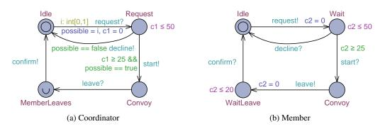
Figure 2.4: Network of Timed Automata Specifying a Simple Convoy Behavior
