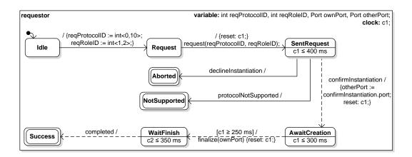
Figure A.24: RTSC Implementing the Role requestor of the RTCP ProtocolInstantiation
