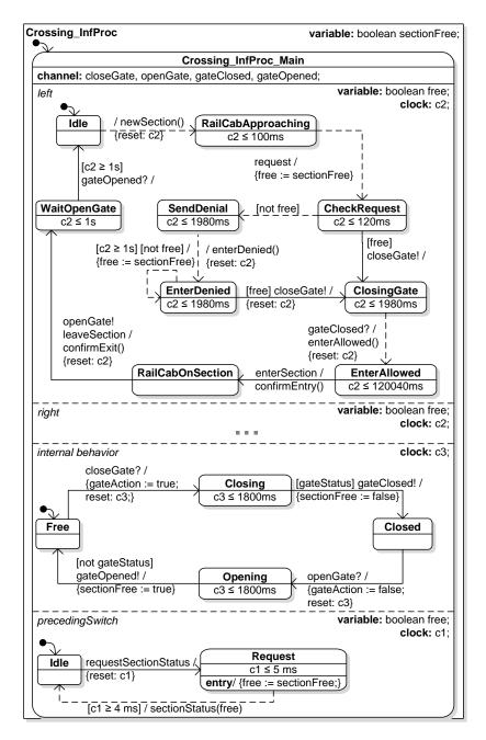
Figure A.41: RTSC of the Component Crossing\_InfProc
