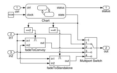
Figure 6.9: Example of a Simulink Model for a Fading Component [Vol13]
