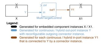
Figure 6.12: Generation Template for Translating Continuous Connector Instances
