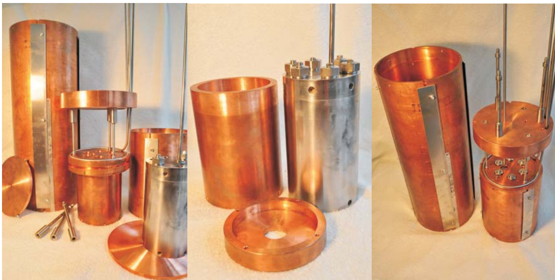
Figure 3.6: (Left) Thermostat consisting of two copper shieldings, each including taps and three distance holders. (Center) Pressure vessel with copper jacket. (Right) Mounted pressure vessel in copper shielding with distance holders and tap for second distance copper shielding.
