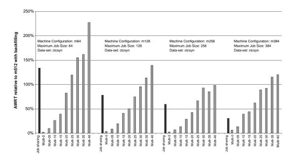
Figure 7.9: Results for different resource configurations compared to configuration m512 with backfilling (equals 0%).
