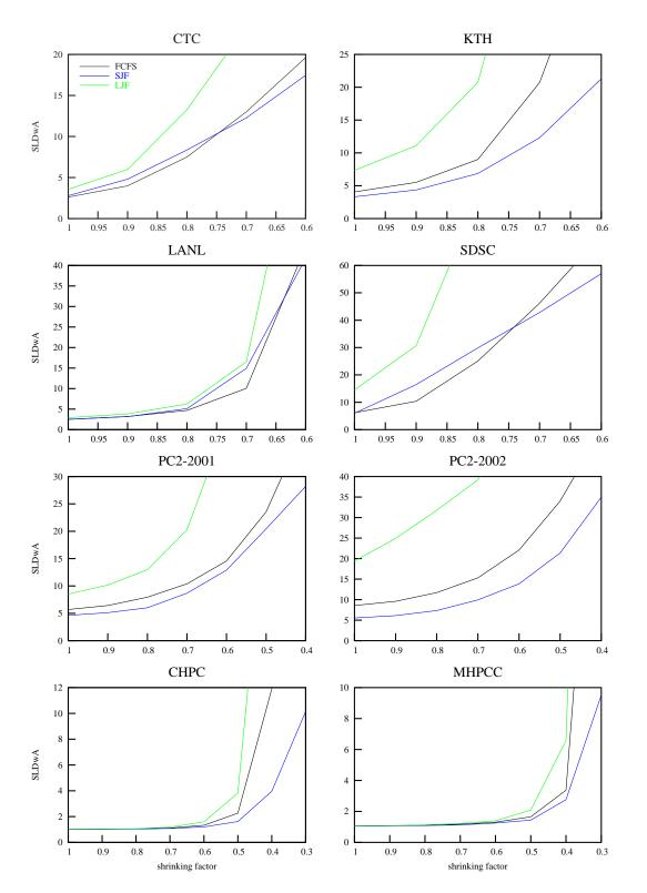
Figure 5.1: Average slowdown weighted by area (SLDwA) of FCFS, SJF, and LJF with different workloads/shrinking factors.
