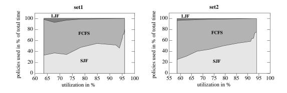
Figure 4.2: Accumulated percentages of policies used by the dynP scheduler with lower bound 7200 s and upper bound 9000 s. set1 left, set2 right.
