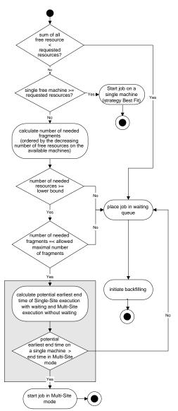
Figure 7.12: Algorithm for multi-site scheduling with constraints.
