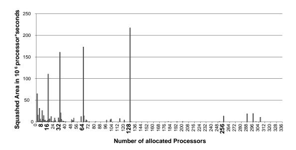
Figure 7.13: Distribution of the resource consumption (or squashed area) in the synthetic CTC workload.
