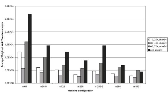
Average Weighted Wait Time in seconds for Job Sharing and all machine configurations and workloads
