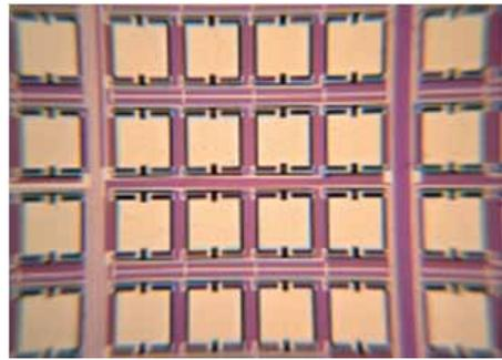
*Micro mirror array for optical applications.*
