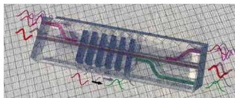
Our goal is to use engineered integrated nonlinear optics to bridge this gap. Special focus lies on the interconversion between the  $\text{Yb}^{2+}$ -transition at 369.5nm and the 1310nm telecommunication window for use in a continuous variable quantum repeater protocol. We employ KTP waveguides, which we only recently added to our fabrication capabilities. With those we aim to reach conversion efficiencies close to unity.
