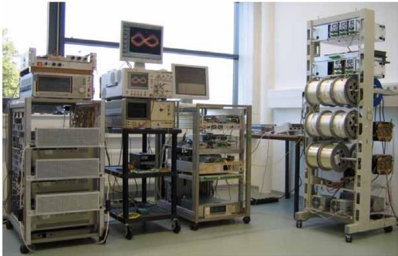
*Using DQPSK combined with polarization division multiplex, we have transmitted 5.94 Tbit/s (5.940.000.000.000 bit/s) over 324 km of fiber in the optical C band alone (world record until 2007).*
