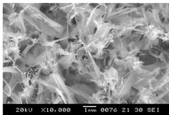
Nanoflakes and nanowires of ZnO seen in an SEM.
