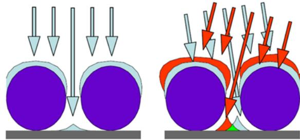
**Cross-sectional view of nanosphere lithography beads used as masks in deposition processes.**
