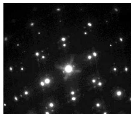
TEM diffraction pattern of an epitaxial 3C-SiC film on silicon.
