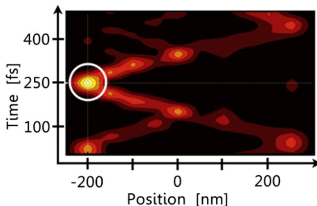
*If the pulse excites a quantum wire, the electrons are concentrated at a desired location in space and time.*
