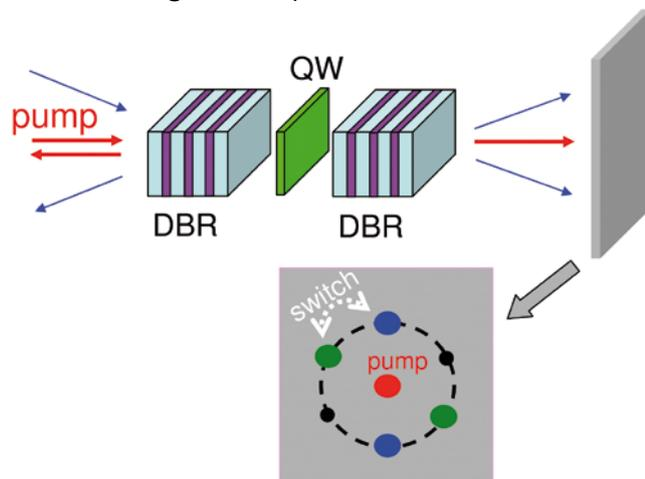
Fig. 1: All-optical switch based on transverse polariton patterns.
