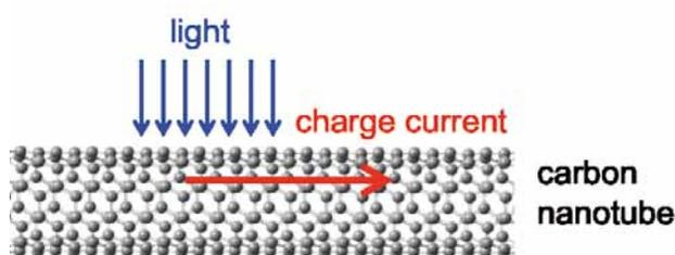
Fig. 2: Photogalvanic effect in a semiconducting carbon nanotube without inversion symmetry.
