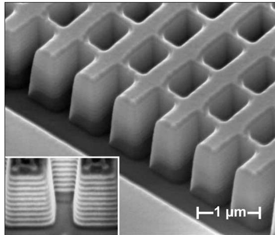
*Metamaterial with a negative index of refraction.*
