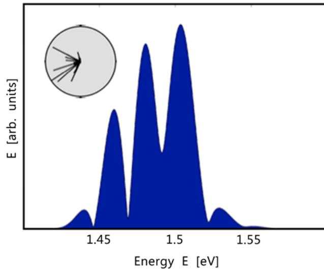
*Spectrum of a laser pulse with the respective phases found by an optimization routine.*
