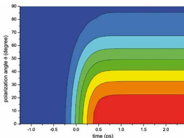
Fig. 3: Photocurrent in a semiconducting carbon nanotube for different angles of incidence for a circularly polarized 1ps light pulse.
