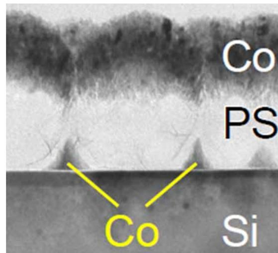
*Cross-sectional TEM micrograph of a polystyrene (PS) mask on silicon, covered with cobalt to create Co nanopylamids.*
