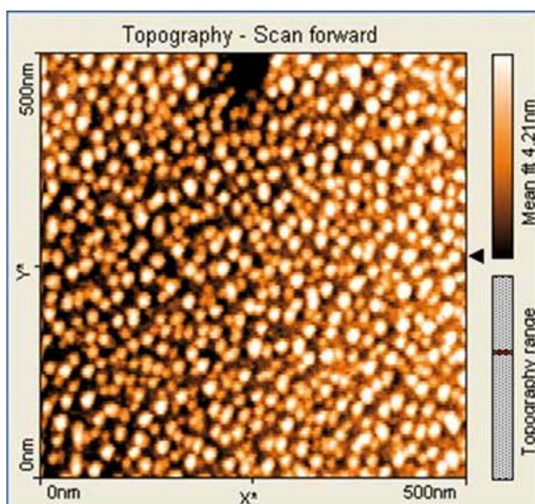
Fig. 2: Atomic Force Microscopy (AFM) image of cubic GaN quantum dots (QDs) on cubic AlN grown by Molecular Beam Epitaxy (MBE) with the Stranski-Krastanov method (area  $0.5 \times 0.5 \mu\text{m}^2$ , density  $5 \times 10^{11} \text{ cm}^{-2}$ ).
