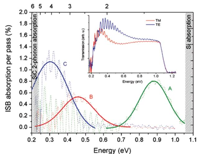
Fig. 1: Transmission spectrum in the THz range of the GaN/AlGaN cubic QWs at 4.2K for TM- (red solid line) and TE- (blue dotted line) polarized light. ISB absorption is peaked at 4.76 THz.
