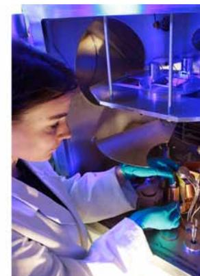
*Luminescent liquid crystals and high vacuum chamber for fabricating thin electroluminescent layers.*
