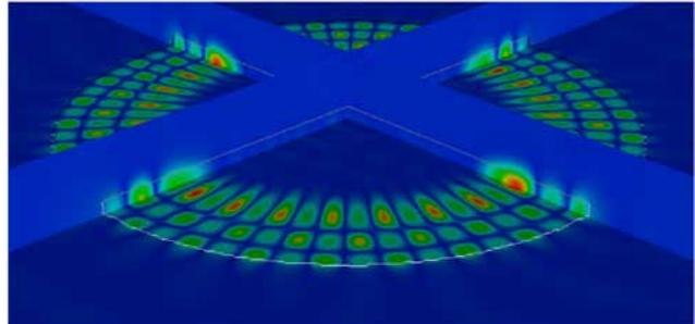
*Whispering gallery mode of a optical micro disk resonator surrounded by a liquid crystal*
