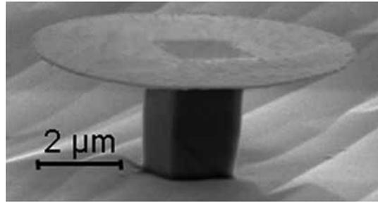
*Low-threshold microdisk laser.*
