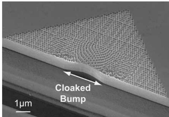
*Optical "carpet" cloak based on nanostructured silicon.*
