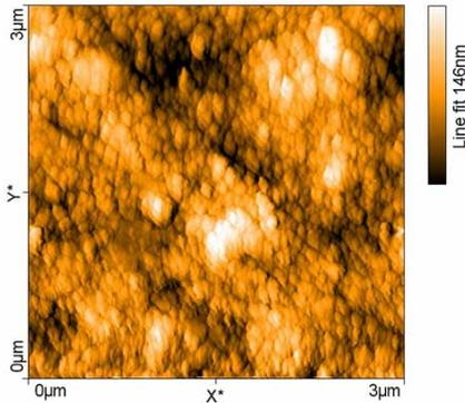
AFM-topography of a silicon nanoparticle surface.
