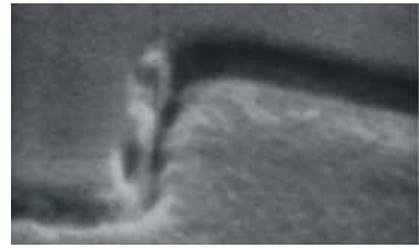
SEM micrograph of an 80nm trench.
