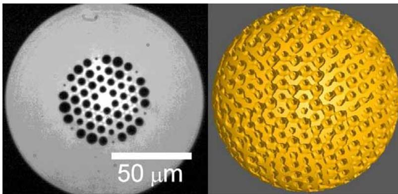
*Cross-section of a photonic crystal fiber (to the left) and three-dimensional structure of a holographic polymer-dispersed liquid crystal.*
