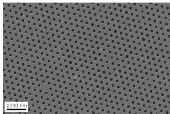
SEM image of an array of subwavelength nanoholes in a metallic thin film formed by NSL.
