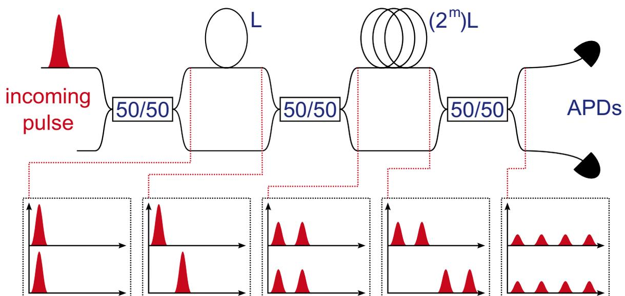
Experimental setup for photon statistics measurement.
