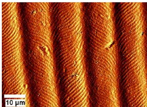
But also dissipative structures caused by electro-convection can be utilized for fabricating regular microstructures: The figure to the left shows the surface shape of a polymer film (detected by atomic force microscopy), where a transient pattern induced by a uniform electric field was permanently imprinted into the polymer surface by means of photopolymerization. The lattice constant of the chevrons is smaller than 1 micrometer.
