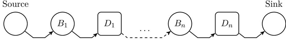
**Figure 8.1:** Sequentially connected generic material flow model  $Q$ .
