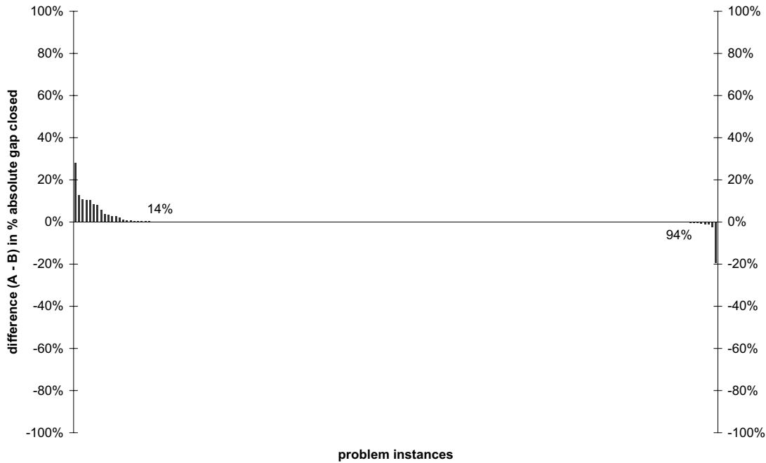
Figure 6.24.: Comparison between a solver version where the uPMC generator and the cMIR cut generator are used (A) and a version where only the cMIR cut generator is used (B). In both cases no cuts are generated out of cuts.
