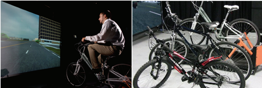
Figure 3-6: Bicycling simulator at the Oregon State University (OSU) [HMJ+15]
