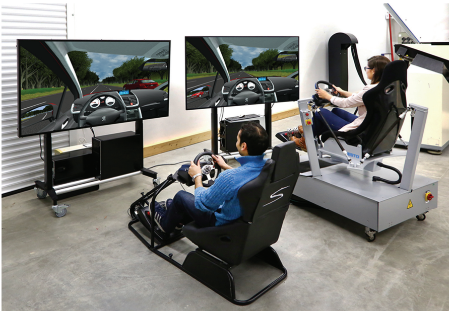
Figure 5-12: Developed platform of networked driving simulation for the second example application scenario
