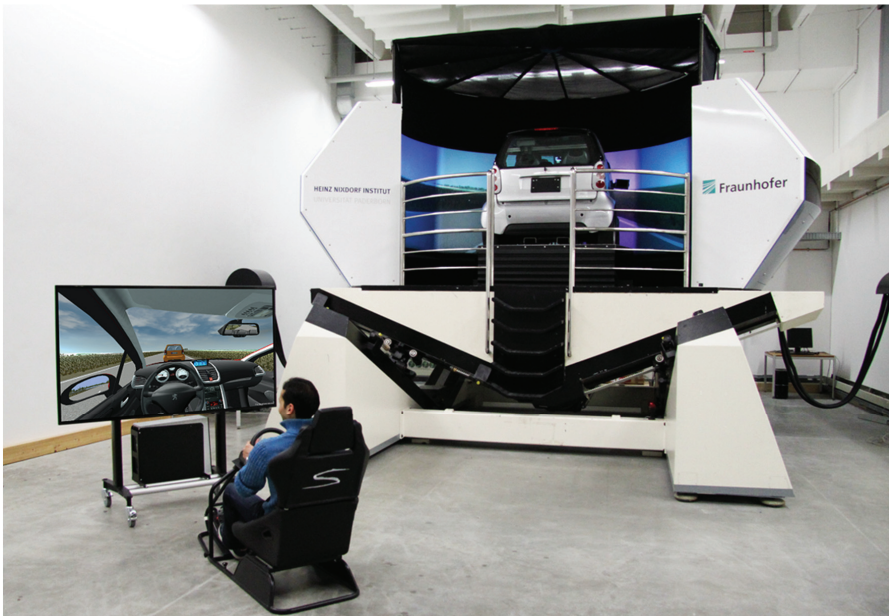
Figure 5-7: Developed platform of networked driving simulation for the first example application scenario
