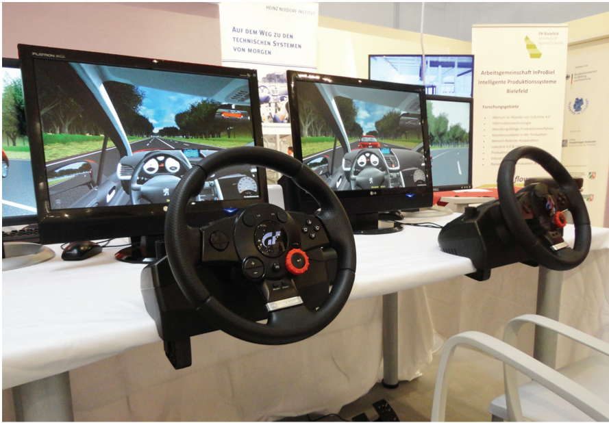
Figure 5-17: Developed platform of networked driving simulation for the third example application scenario
