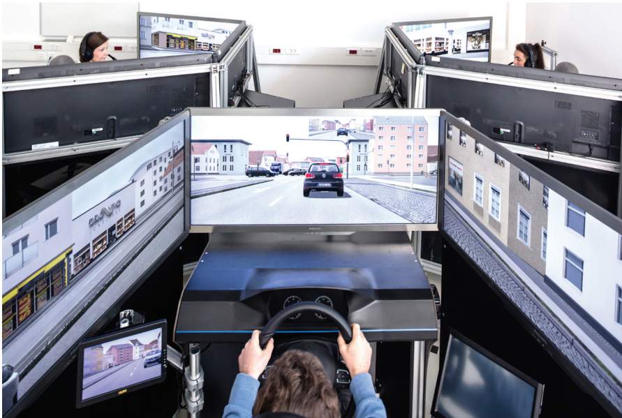
Figure 3-3: Multi-Driver Simulation Lab at the Institute of Transportation Systems, German Aerospace Center (DLR) [OS15]
