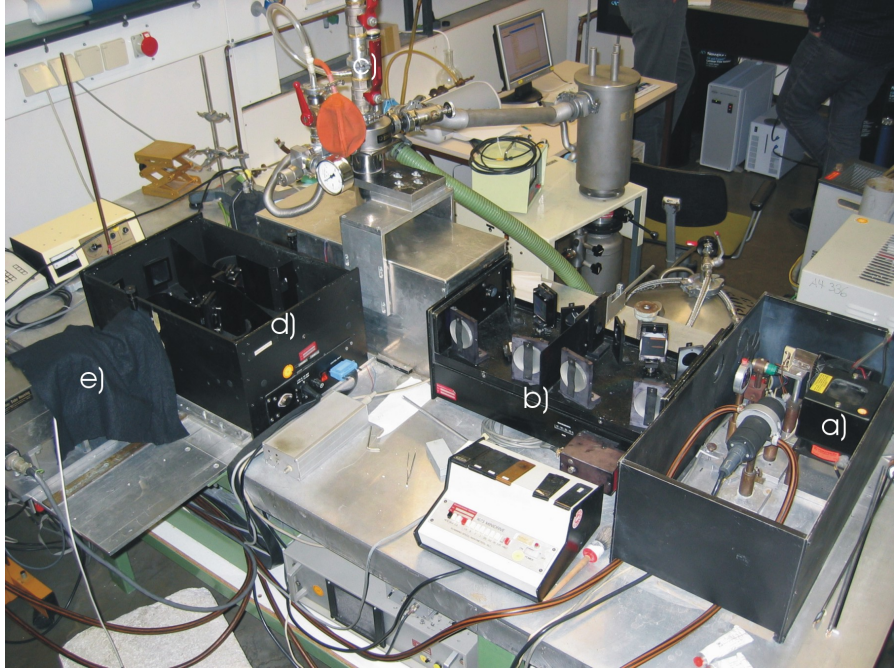
Figure 2.5: Photograph of the luminescence spectrometer: a) Xenon lamp, b) excitation monochromator, c) cryostat, d) emission monochromator, e) Photomultiplier.
