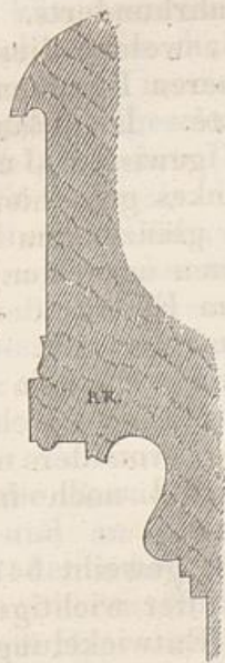
Grabmal Theodorichs, Kranzgesims.
