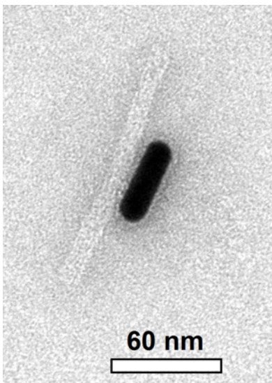
Gold nanorod on a DNA origami nanostructure [TEM, recorded by Bingru Zhang]. Right: Cromoglycate needles induced by DNA nidi decorate a LC [polarisation-optical micrograph, scale bar: 200 \mu\text{m} ].
