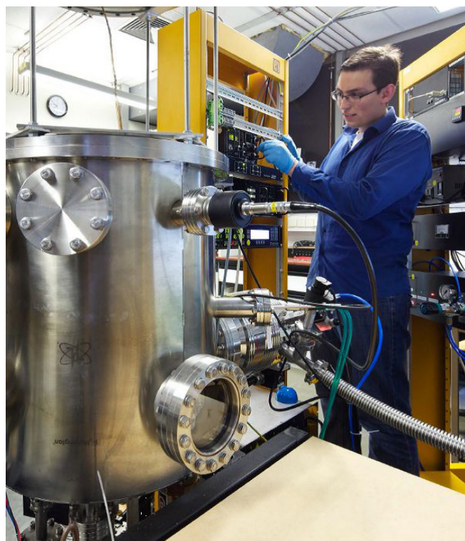
Home-built electron beam evaporation system dedicated to the large-area fabrication of arrays of geometrically and chemically tailored plasmonic nanoparticles.
