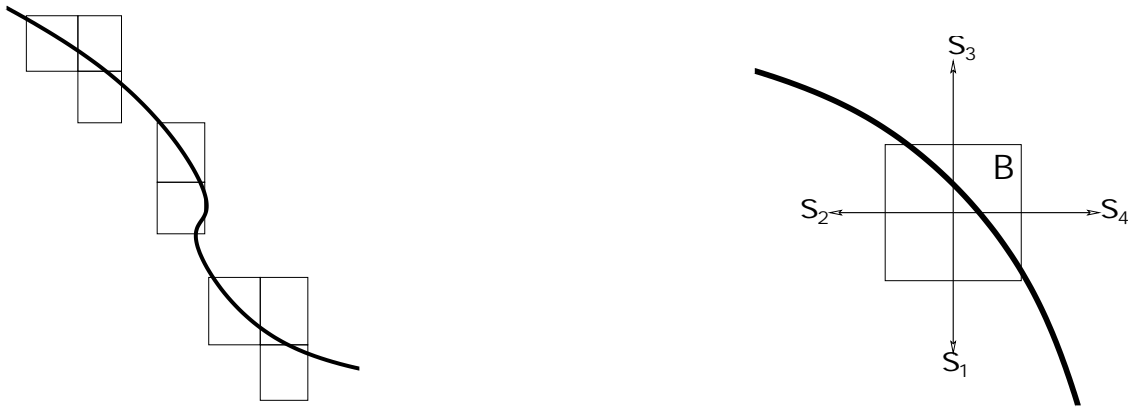
Figure 6.5: Recovering algorithm: uncomplete covering of the Pareto set (left) and possible choice of test points for a given box B (right).
