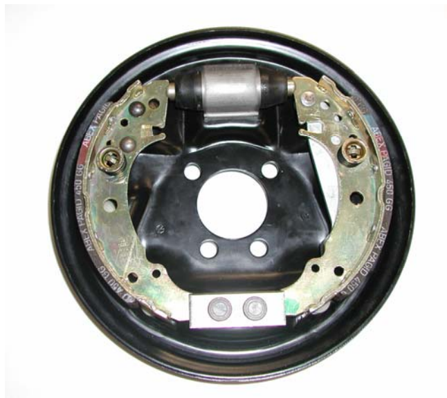
Fig 6.1 Sliding simplex drum brake [VW-GOLF II]
