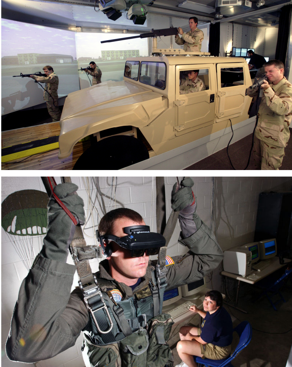
Figure 2-6: Military virtual reality applications: Virtual Combat Convoy Trainer (up) and Virtual Reality Parachute Trainer (down)
