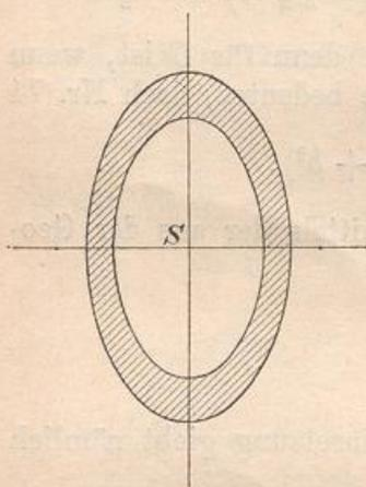
$$T_1 = \frac{a_1^3 b_1 \pi}{4} - \frac{a_2^3 b_2 \pi}{4} = \frac{\pi}{4} (a_1^3 b_1 - a_2^3 b_2).$$
