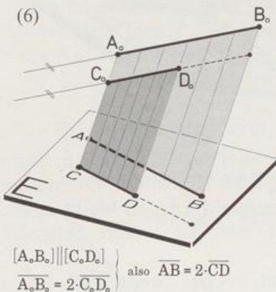
$$[A_0B_0] \parallel [C_0D_0] \quad \left. \begin{array}{l} \\ \end{array} \right\} \text{also } \overline{AB} = 2 \cdot \overline{CD}$$
