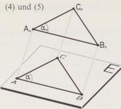
Ebene( $A_0B_0C_0$ )  $\parallel$  E also  $\triangle A_0B_0C_0 \cong \triangle ABC$
