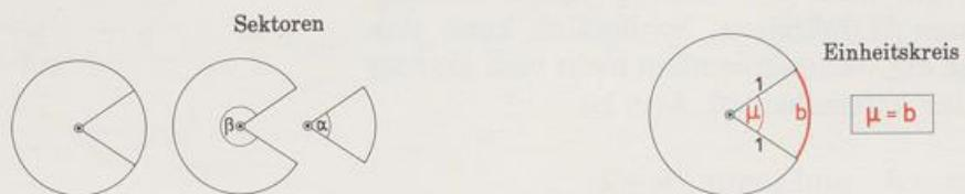
$$\frac{b}{2r\pi} = \frac{\mu}{360^\circ} \quad \text{und damit} \quad b = 2r\pi \cdot \frac{\mu}{360^\circ} = r\mu \cdot \frac{\pi}{180^\circ}$$
