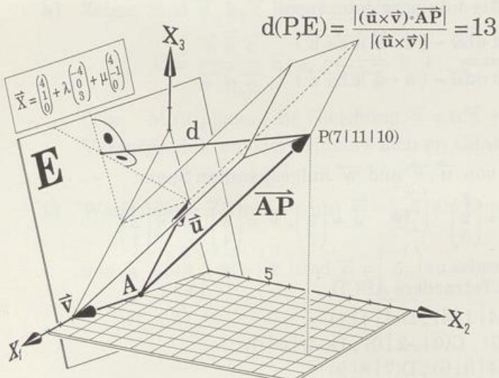
$$d(P,E) = \frac{V}{G} = \frac{|(\vec{u} \times \vec{v}) \circ \overrightarrow{AP}|}{|\vec{u} \times \vec{v}|}$$
