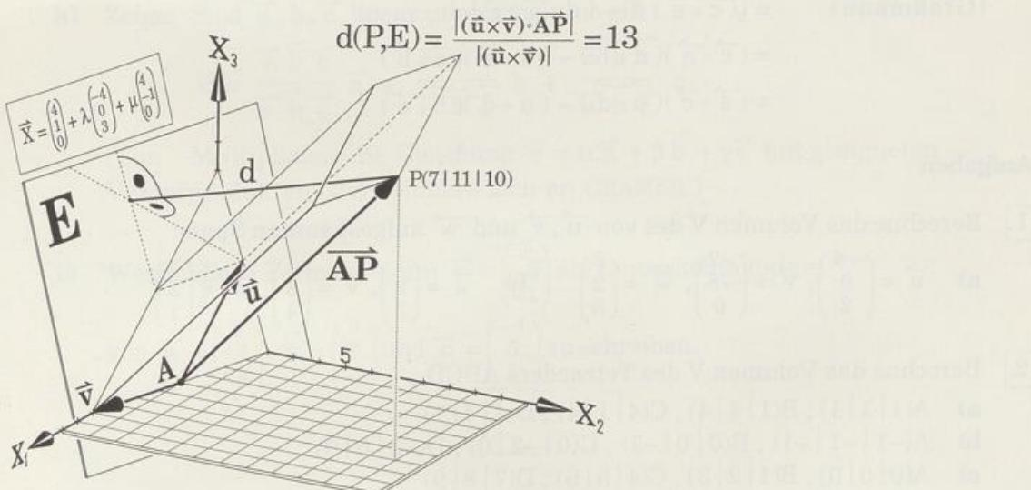
$$d(P, E) = \frac{V}{G} = \frac{|(\vec{u} \times \vec{v}) \circ \vec{AP}|}{|\vec{u} \times \vec{v}|}$$
