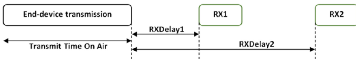
Figure 2.2: LoRaWAN Communication for Class A devices (Mekki et al., 2019)
