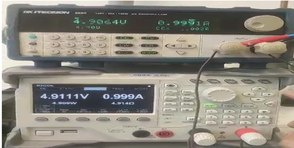
Figure 4.19: Variable electronic Load and Programmable DC Supply used at the laboratory
