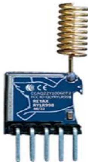
Figure 4.13: RYLR 998 LoRa Module source: (LoRa Datasheet, (2021))
