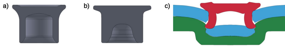
Fig. 7 a Rivet geometry of the multi-range capable rivet (K-rivet), b Rivet geometry of the HDZ rivet, c Numerically determined failure behaviour of the K-rivet for the material combination CP1000 in 1.5 mm sheet thickness in EN AW-6014 in 2.0 mm sheet thickness
