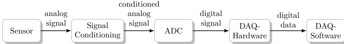
Figure 5.9: Typical measurement chain for sensors
