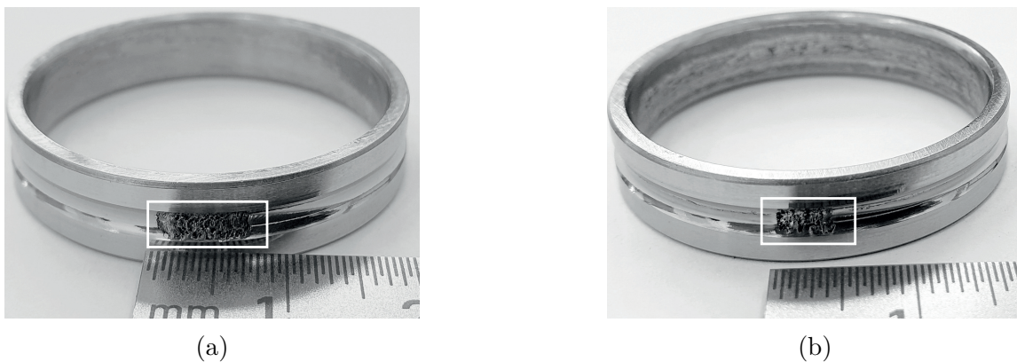
Figure 5.18: Spalling on the inner raceways of the test bearing after the experiment: (a) B02 and (b) B03
