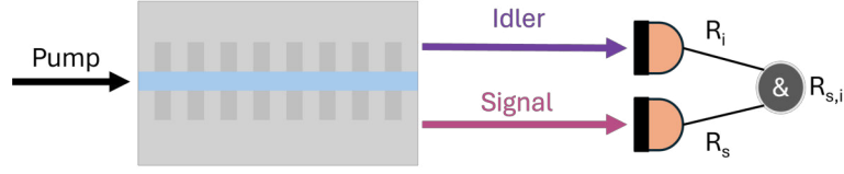
Fig. 2.19: Measurement scheme to evaluate the Klyshko efficiency.
