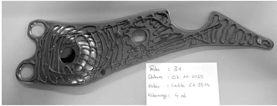
Figure 7.32: Adhesive applied to the lower 1.2 mm patch for specimen B1. 0.2 mm steel spacers can be seen embedded within. The amount of glue is 4 ml, corresponding to an overall bonding thickness of 0.2 mm with a 100 % surplus to fill any possible gaps larger than 0.2 mm, e.g. in tight radii.
