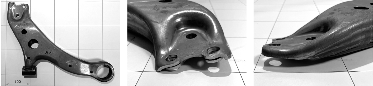
(a) Specimen A7, 3 mm base thickness without patch, after static testing with 25 mm deflection.
