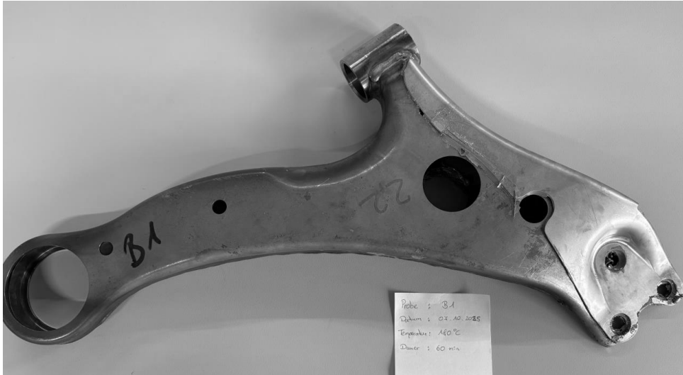
Figure 7.34: Wishbone link prototype after curing.
