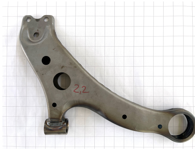
Figure 7.30: Wishbone link after OP2.2 welding, 2.2 mm variant.
