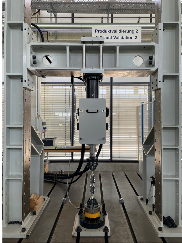
Figure 6.5: Hydraulic universal test bench for performing the pulsating fatigue testing of adhesive specimens with the specimen clamping rig mounted to it. Force is exerted by the vertical hydraulic piston above the rig and measured by a pressure sensor below it.
