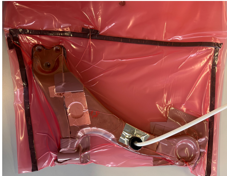
Figure 7.33: Wishbone link adhesive curing set-up.
