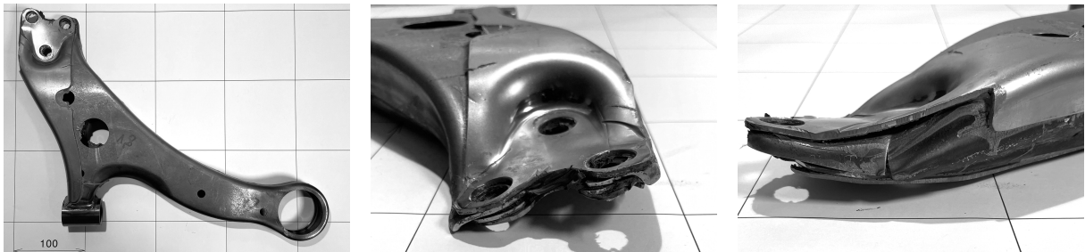
(c) Specimen C1, 1.8 mm base thickness with 2.2 mm patch, after static testing with 35 mm deflection.
