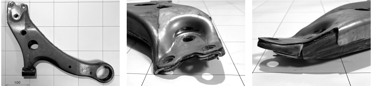
(b) Specimen B1, 2.2 mm base thickness with 1.2 mm patch, after static testing with 35 mm deflection.
