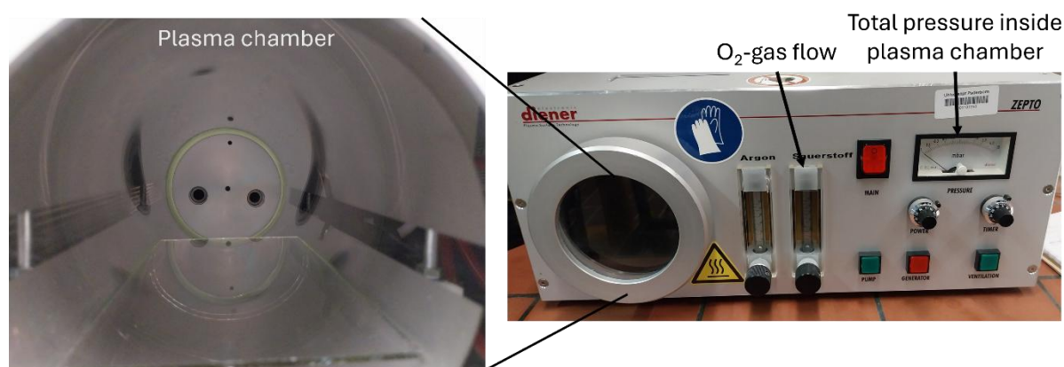
Figure 21. Photograph of the plasma generator used in this thesis. The left image shows the plasma chamber including the glass slide support for the samples. The right image shows the plasma generator with the \text{O}_2 gas flow and total pressure displays indicated.
