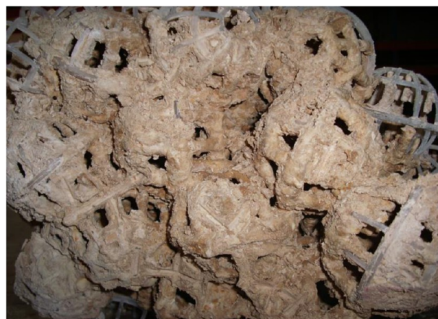
Figure 18. Solid residue on conventional random packings leading to clogging of the column during ammonia stripping from agricultural waste. Photo by ENVIMAC Engineering GmbH.
