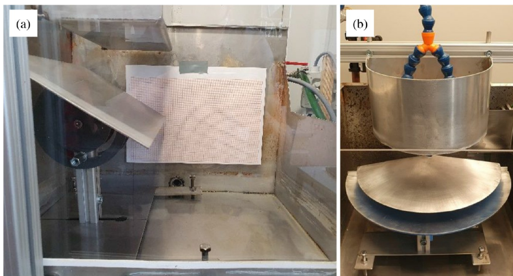
Figure 3. View through the window of the experimental setup onto the plate (a) 15 and adapted layout with CAF inside the reservoir (b) (Reproduced from S.A. Bernemann et al, Chem. Eng. Sci. , 2024 , 300, 120639, under the terms of the CC BY-NC-ND 4.0 license).
