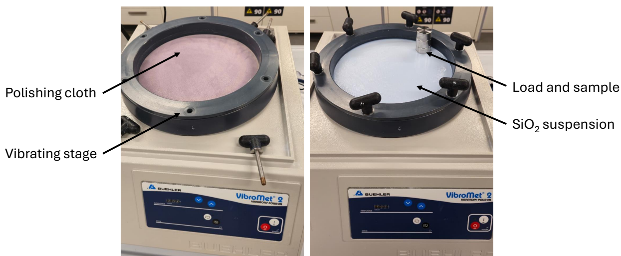
Figure 3.6. Vibratory polishing machine with the vibrating stage and polishing cloth (left). The image on the right shows the polishing process, where the loaded sample with weights rotates in a \text{SiO}_2 colloidal suspension on the polishing cloth.
