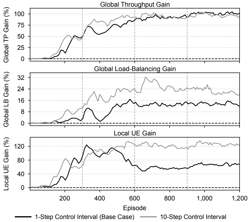
Figure 6.6: Multi-agent training dynamics under reduced control frequency. The curves compare the 1-step base case against a 10-step control interval across training episodes, reporting global throughput gain, global load-balancing gain, and local UE gain, demonstrating how slower updates influence convergence and objective trade-offs. Metrics are smoothed using a rolling mean over a 25-episode window. Reprinted from [35], © 2026 IEEE.
