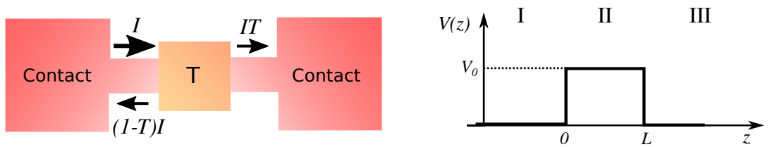
Figure 2.3: Left: System with a scattering region in which a current I is transmitted with a probability T and reflected with a probability (1 - T) . An example for a simple scattering region is a potential barrier ( right ).
