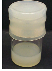
Figure 2.5. Liquid crystal mixture MLC2048. The white color originates from light scattering due to differently aligned liquid crystal domains.
