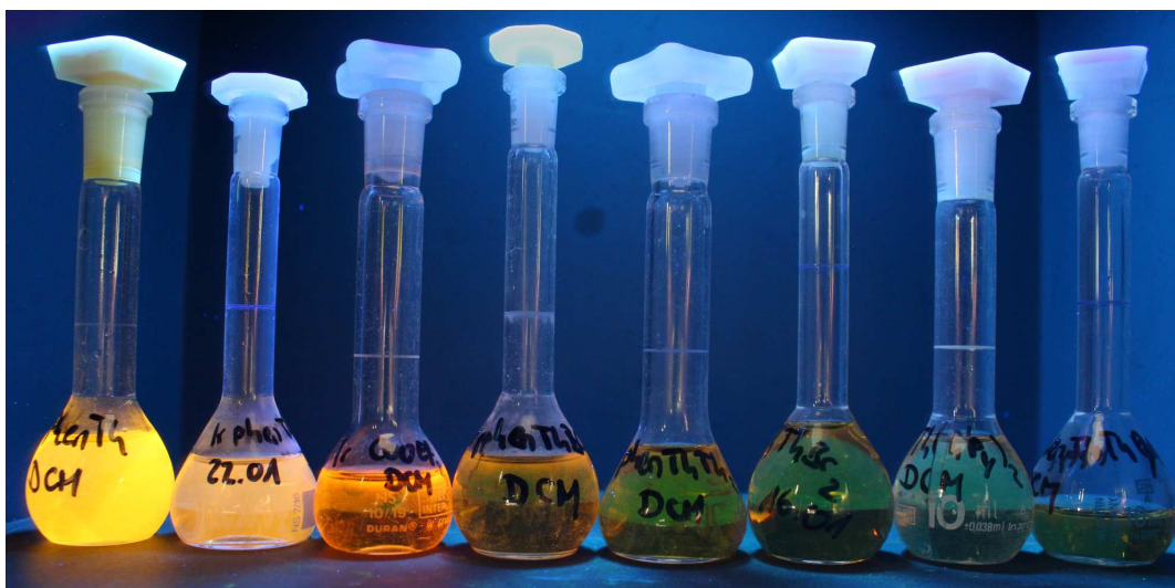
Figure 4.16: Photograph of all synthesized iridium complexes dissolved in \text{CH}_2\text{Cl}_2 under irradiation with UV light. From left to right: PS2 , PS4 , PS3 , PS5 , PS6 , PS7 , PS8 , and PS9 .
