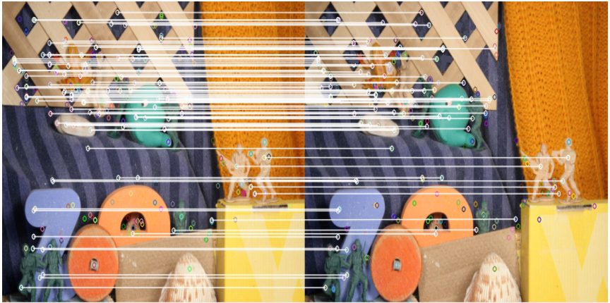
Figure 3.3: Feature points correspondences between two consecutive frames applied on the "Army" sequence from the Midellburry dataset. Here we used the modified census transform MCT as an example to calculate matching correspondences between feature points.
