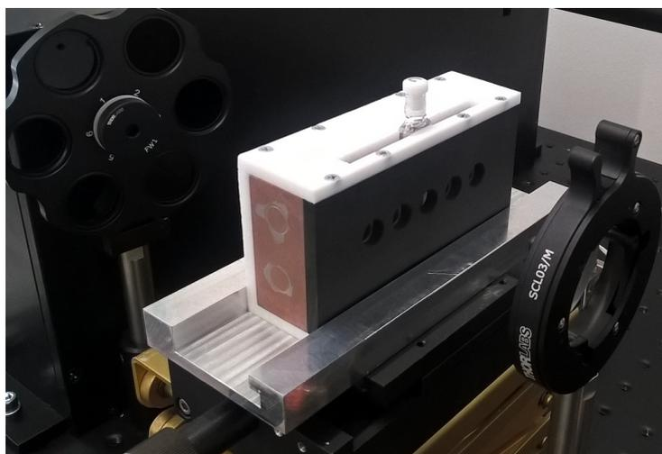
**Figure 3.4:** Stage for liquid samples to enable SALS measurements of colloidal systems hosting up to five flat-cells for investigation of colloidal suspensions. The (attenuated) laser beam enters the stage from the upper left of the image and leaves it together with the forward scattered light to the lower right towards the detection optics. Temperature-control was realized by a water thermostat.
