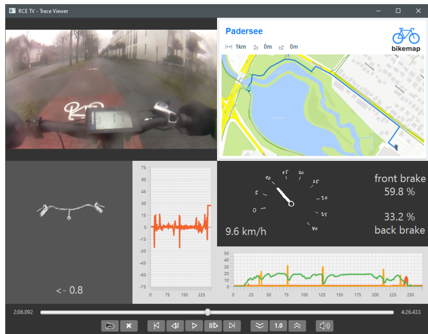
Figure 6.5 – Screenshot of the RCE TV during playback of a recording. The screen is split into four parts, showing the video, the GPS track on a map, the current steering angle, and current speed and brake values. The bad video quality is caused by slight rain during the recording. On the bottom of the video frame, the current speed (e-bike engine) is displayed. In the shown scene a harsh brake maneuver was performed which also can be seen by the high brake values (displayed on the right). Using the video it is clearly visible that the speed reduced radically. The e-bike display, however continues to show the previous speed, i.e., 17.1 km/h. The RCE's speed sensor detected the speed reduction and shows a velocity of 9.6 km/h. Next to the handlebar symbol (bottom left) the steering angle during the entire recording is shown in a line chart. Speed (green) and brake application (orange and red) of the entire recording are shown in the second line chart (bottom right). The control bar can be used to control recording playback, skip single frames back or forth, or change the playback speed.
