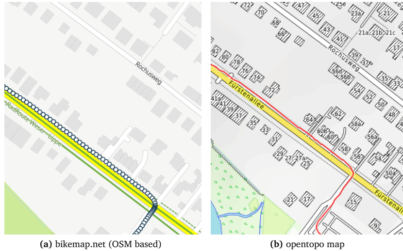
Figure 5.11 – Comparison of two maps with different road width. The track is drawn as dots and as a red line, respectively. Driving direction is starting at the bottom, going to the top left. In (a) the yellow road is drawn with two lanes, one in each direction, so it looks like the track is positioned on the right side of the right lane. In (b) the road is drawn thinner and the track is positioned besides the road.
