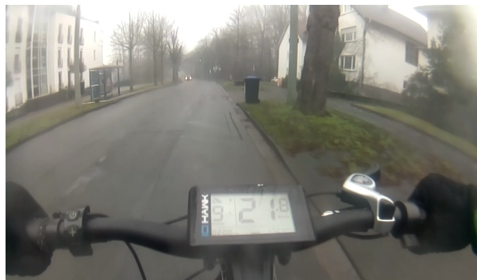
Figure 5.2 – View of the Raspberry Pi Camera during a ride. In the bottom, the display of the e-bike can be seen. It shows the current speed, 21.8 km/h.
