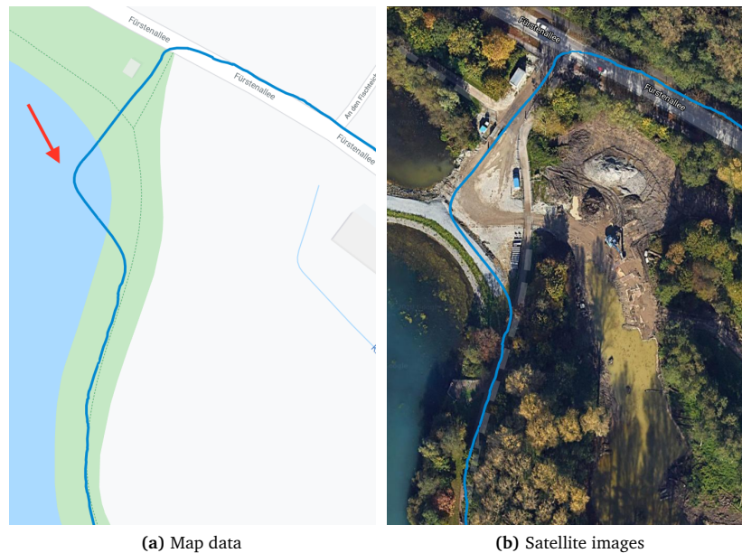
Figure 5.10 – GPS track (blue line) on Google Maps. (a) The map data is outdated and does not yet contain the new path, so it looks like the track goes through the lake at the spot, marked with a red arrow. On the satellite images (b) the construction site can be seen.
