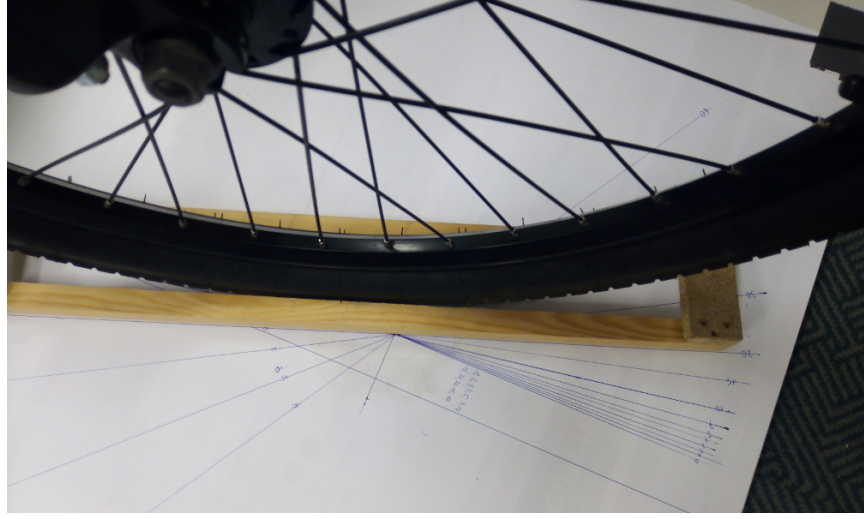
Figure 5.6 – The wooden frame that fits over the front wheel gives a sharp line indicating the angle of the front wheel on the ground plank. Both wheel and frame hover a few millimeters above the plank to avoid friction. In this image, the angle is adjusted to 20^\circ .
