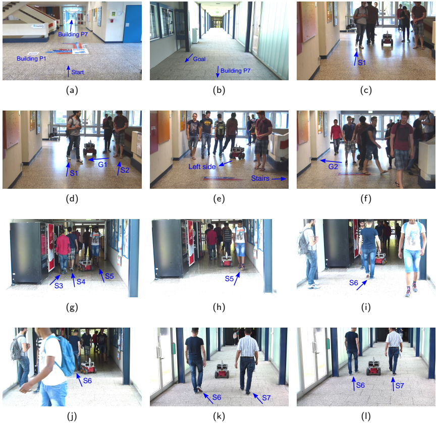
Figure 6.15: Experiment 7. (a, b) Environmental setup, the robot had to move through the connection between buildings P1 and P7. (c-l) Snapshots of the experiment taken at different locations, showing that the robot was able to react on time avoiding the students who stepped in to close its way to the goal.
