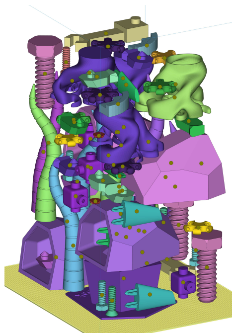
Fig. 2.8 Example for the digital preparation of a SLS build job.
