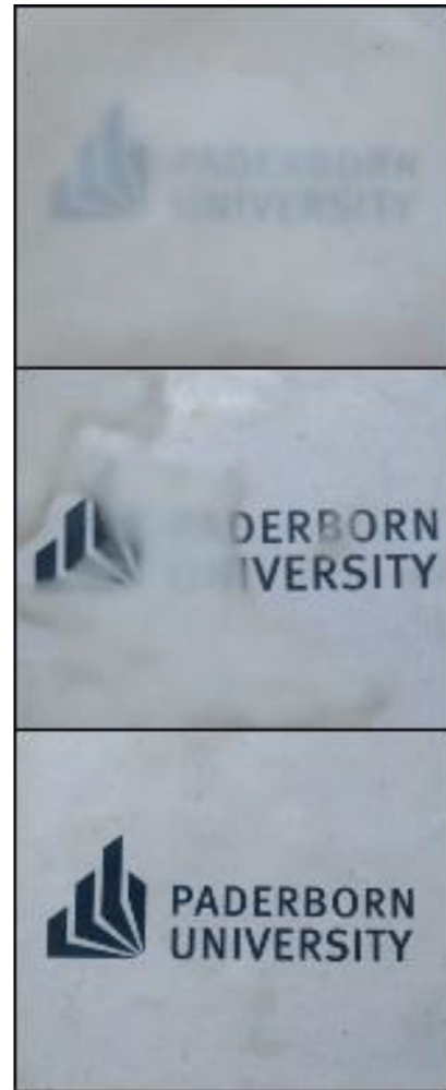
Fig. 4. Transparency of the present polymer compound from solid (top) to liquid (bottom).
