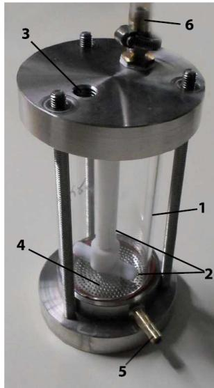
**Figure 87:** Photograph of the Ultrafiltration Unit
