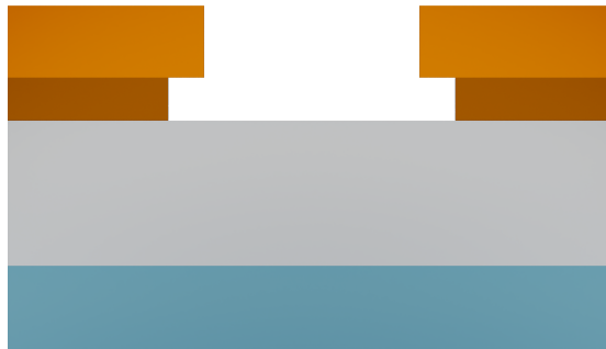
Figure 5.41 – Illustration of a cross-section of the two resist layers and undercut for the lift-off after development.
