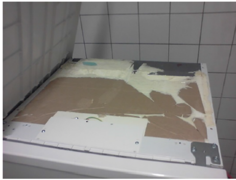
Fig. 8. Missing diffusion barrier at the cabinet of appliance F01.
