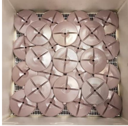
Figure 5-8: First two layers of heatSel arrangement inside the cuboid storage tank [108]
