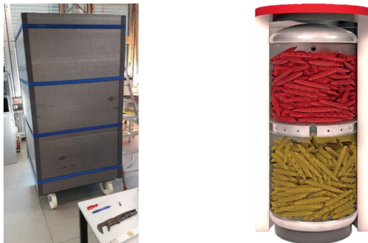
Figure 5-6: Cuboid storage tank (left, [108]) and a PBLHS filled with cylindrical heatStixx (right, illustration by Axiotherm GmbH [111])
