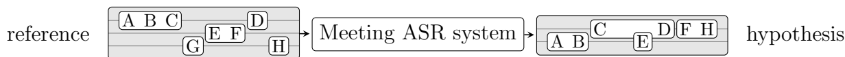
Figure 3.6: An example input and output transcript of a meeting transcription system. Each box represents an utterance and each letter a word. Timestamps are indicated with horizontal position, where time flows from left to right. This example will be used to show how the different WERs solve the assignment problem. (Taken from [OC8])
