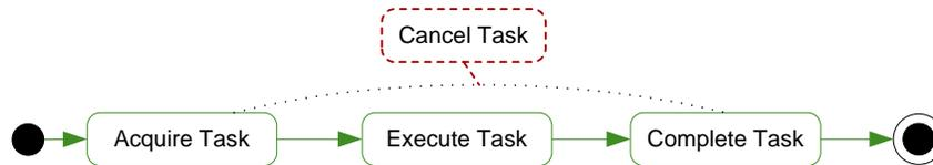
Figure 3.3.18: A forbidden guard spanning multiple situations
