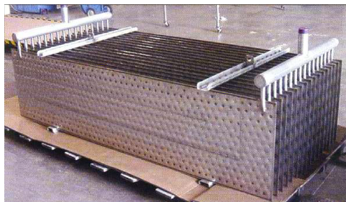
Figure 2.3: Thermoplate assembly (OMEGA heat transfer technology [66]).
