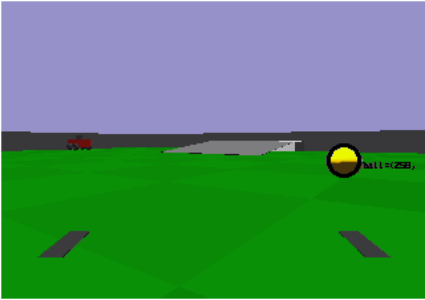
Figure 8.5: The subjective perception of the robot used in the experiments. It shows one camera image with the ball that has been recognized by the vision preprocessing step.
