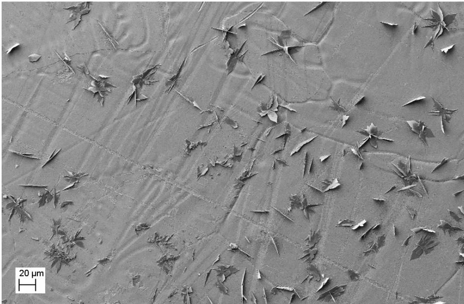
*Fig. 3.19: SEM image of zinc phosphated HDG steel in a standard zinc phosphating bath ( $H_3PO_4$  25 mmol/100 mL; ZnO 1.6 mmol/100 mL) at 60°C and p hosphating time of 60 s.*
