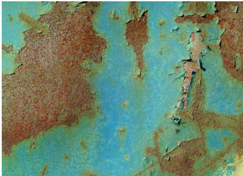
*Fig. 1.1: Example of corroded steel surface where the coating has lost its ability to protect the surface from oxygen and humidity [1].*
