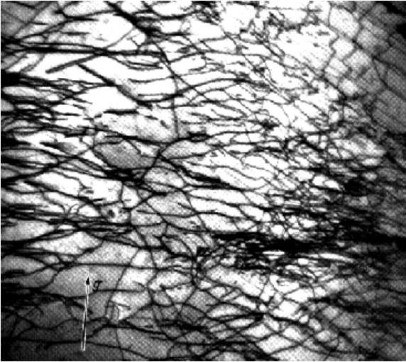
Figure 1.17: Dislocations in Stage II for a f.c.c. Ni+40%Co alloy. The glide direction is denoted by g : the majority of the primary dislocations are edge dislocations. In the upper right corner there are dislocations drawing an angle of 30^\circ with the primary ones. They are the dislocations formed along the intersection line between the primary and the conjugate plane. Glide=0.70. After [67].
