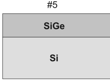
Figure 5.5: Schematic illustration of the vertical structure of sample #5.
