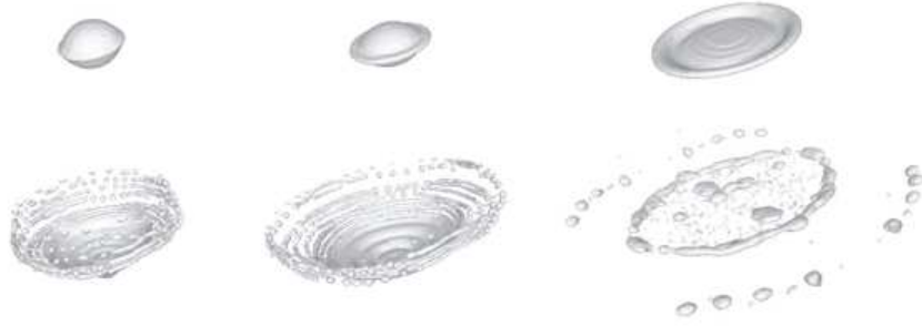
Figure 5.8.: Sequence of simulated deformations of a water drop with kR_s = 0.3\text{mm} .
