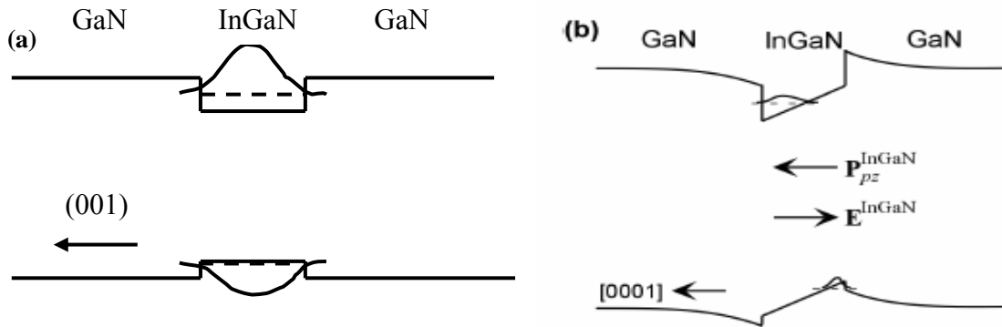
Figure 4.4 The band profile and carrier distributions in cubic and hexagonal InGaN/GaN quantum well, a) the cubic InGaN/GaN DH structure, b), the h-InGaN/GaN DH structure.
